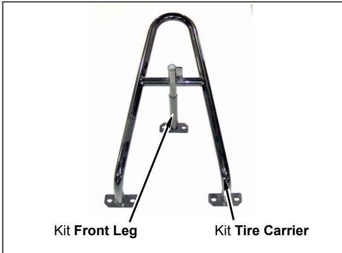
2. Secure kit **front leg** to kit **tire carrier** with kit **bolt** (3/8" x 1") and kit **washer** (3/8" USS).
